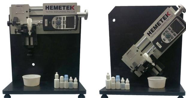
At the heart of the squeeze force testing system was the digital Chatillon DFS II force gauge that features a simple user interface, large full color display and offers accuracy better than 0.1% of full scale. Loads are displayed in ozf, gf, lbf, kgf and N units.
