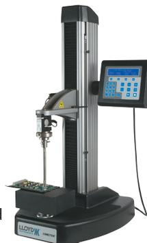
Instruments was used in combination with a 100N YLC load cell, a splinter shield with inlock, the NEXYGENPlus software with a special script and RS232 controllers.
